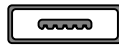
Figure 4.6. USB Series Micro-AB Receptacle for USB OTG Dual Role Devices only. Even smaller form factor.
